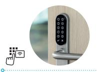
SMARTair escutcheons are available with an optional integrated keypad for multi-factor authentication and convenience. Open with a PIN, your RFID credential, a combination of RFID + PIN for an extra layer of security, or a smartphone with the Openow app.
